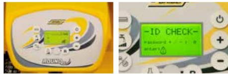
Control panel with display. Access password (it can be enabled on demand)
